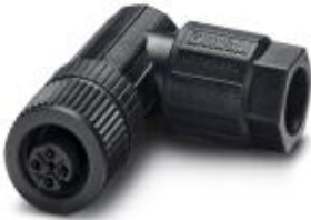
Connector, 4-position, Socket angled M12, A-coded, Spring-cage conn., Knurl material: Plastic, External cable diameter 4 mm ... 8 mm
